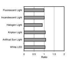
Fig.2 Light Source Dependency (Fluorescent Light is set to '1')
