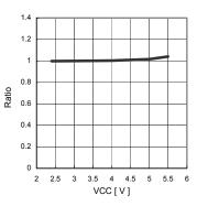
Fig.9 IOUT VCC dependency
