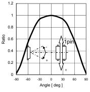
Fig.5 Directional Characteristics 2
