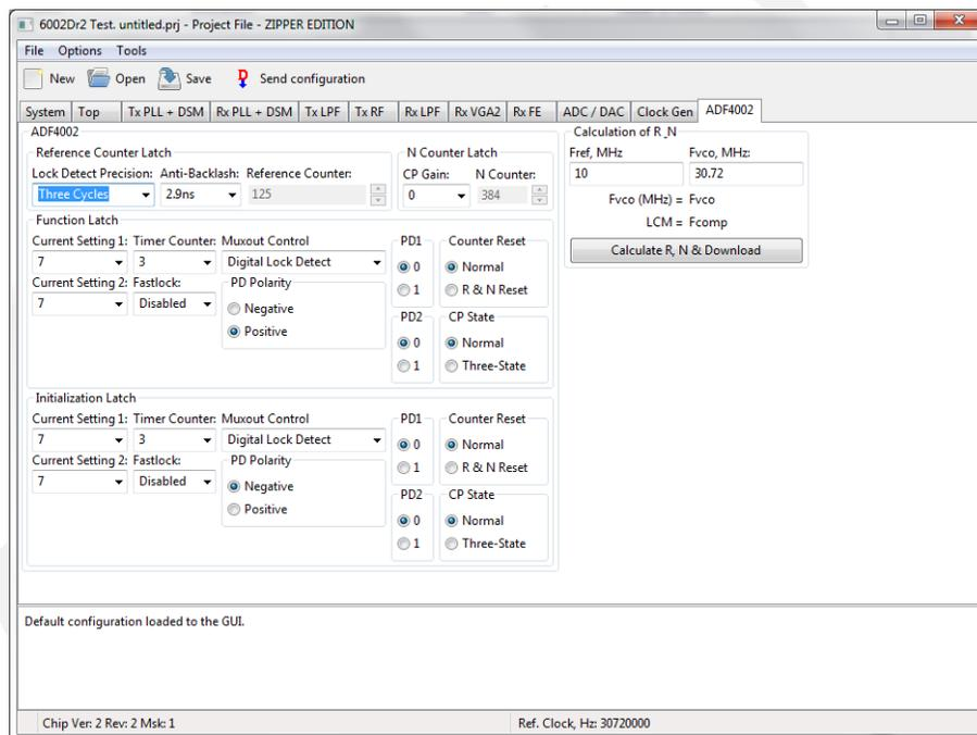
Figure 28. Control window for on board ADF4002.
