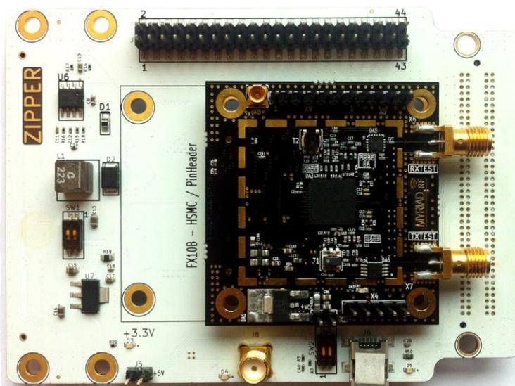
Figure 1. Zipper and Myriad-RF board development system
