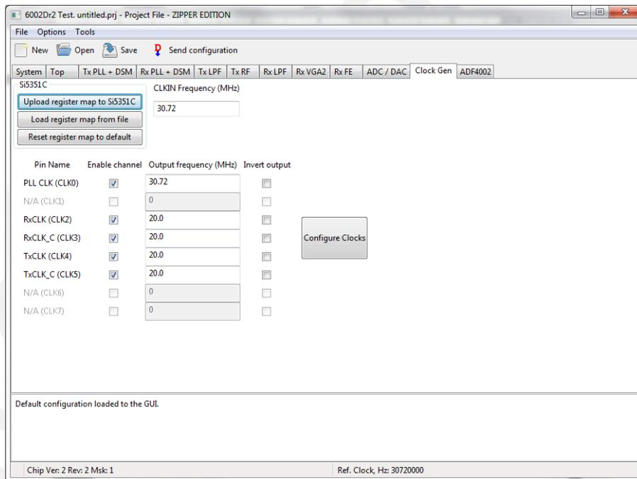
**Figure 27. Control window for on board clock generator.**
