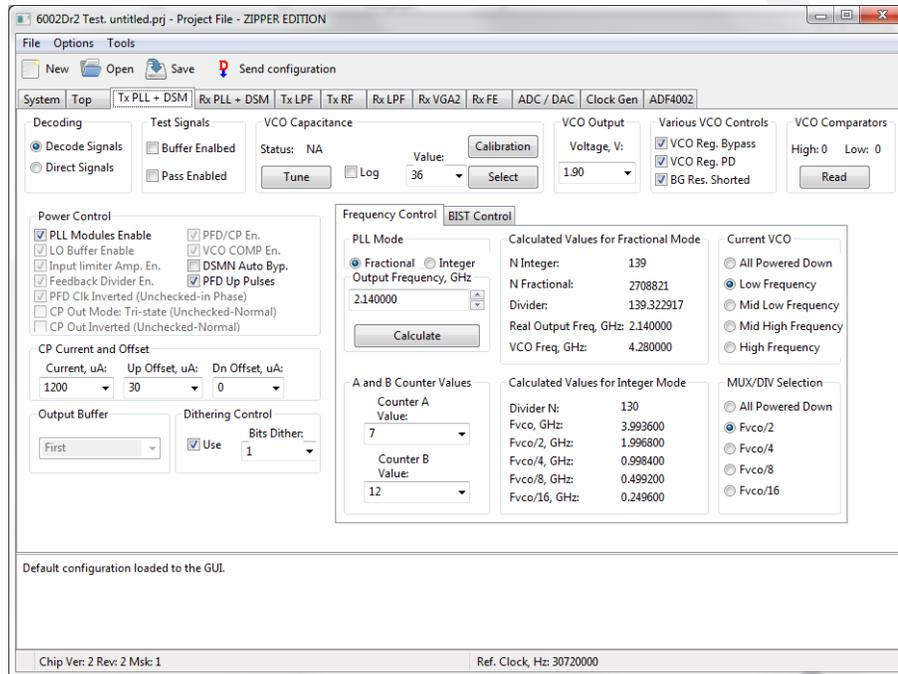
Figure 15. Zipper software TxPLL + DSM window
