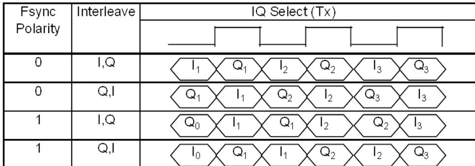
Figure 25. DAC enable control timing for TX
