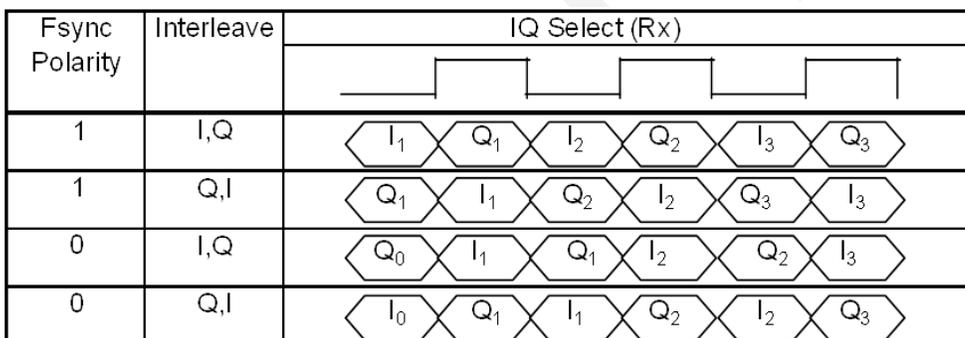
Figure 26. ADC enable control timing for RX
